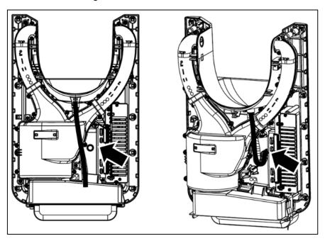
Fit the hose supplied with the machine to the water drain at the rear of the machine. Mount the machine on the wall keeping in mind that the hose mounted on the machine must enter the drain in the wall.
